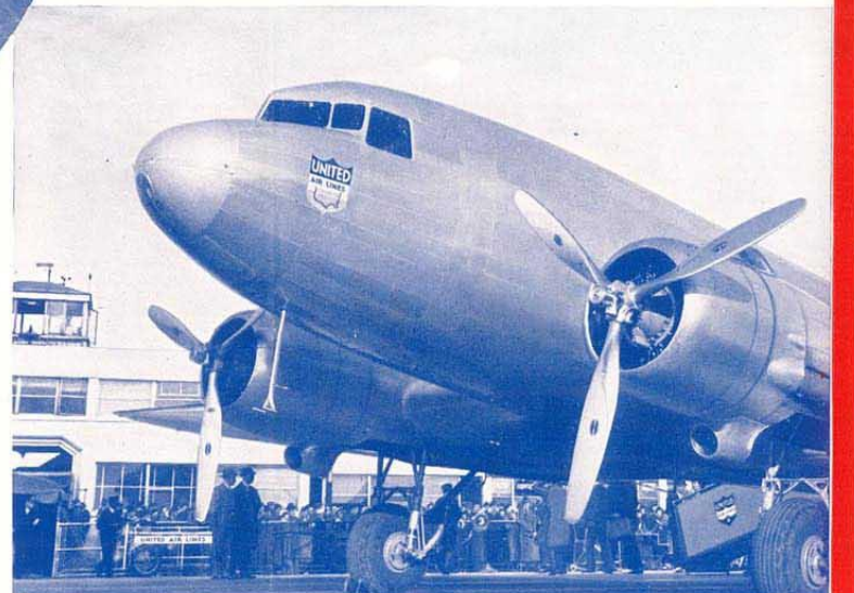
FLYING AIDS—Nation's Most Powerful Land Plane . . . Latest multiple radio navigation . . . Constant speed propellers . . . Automatic gyro pilot . . . De-icers on wings and propellers . . . 1937 type instruments . . . 100 million miles experience.
