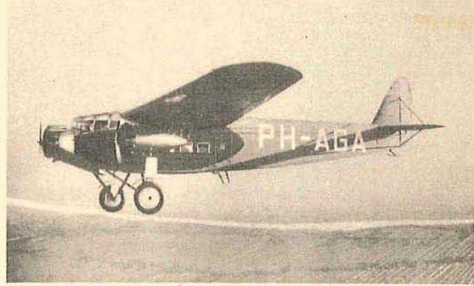
FOKKER F IX Three engined K. L. M. Air Liner accommodating 18 passengers and two Pilots
