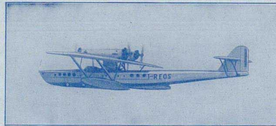
Four-engine Dornier-Superwal Flying Boat in service on the Genoa-Barcelona line entirely metal-built - 2 passenger cabins - 20 seats
