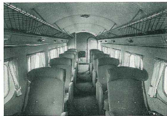
Every passenger seat on the Bloch 220 is against a window. Individual ventilation and light controls are above each seat.
