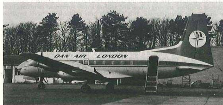
The Hawker Siddeley 748 has been specially designed for short-range flights. It has an out-standing record of reliability and is powered by two Rolls-Royce Dart engines. This modern aircraft is fully pressurised for passenger comfort and has a seating capacity of 48.
